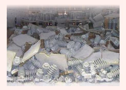
Since the kiln is not an airtight vessel and has no internal pressure, no explosion had taken place. The blast of unburnt gas in the form of a cloud which had remained at the rear side of the kiln had caused the damage and according to him, was not an explosion under the policy. The subsequent damages to the kiln refractory had occurred due to shock waves which might have been created due to gas cloud burst, which does not come under the policy coverage.
