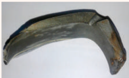
Close-up View of the Pressure side of the Fractured Turbine Blade
