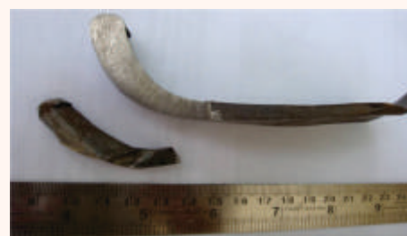
Cut-away view of the samples sent for Lab analysis, sheared in way of DW hole towards the leading edge
