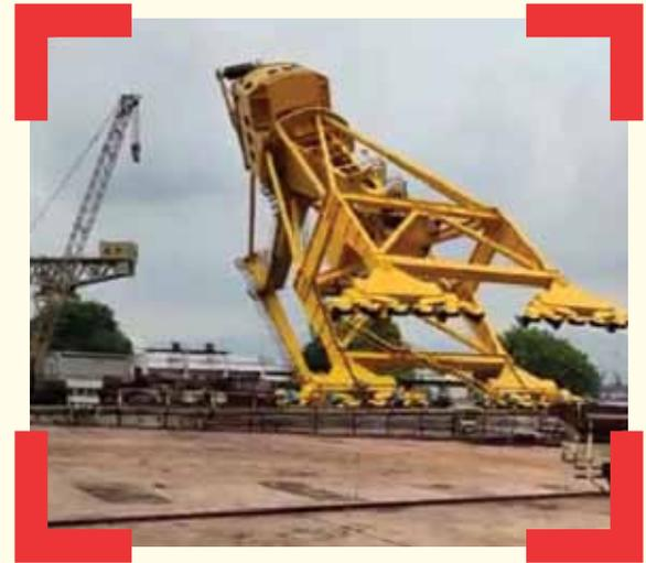
The company did not provide a design manual for the crane, the panel found, and added that four bearings, including central bearings, were damaged, triggering the collapse.
